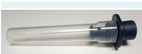
FIGURE 1. View of a Net Bio BioChipSet swab.
